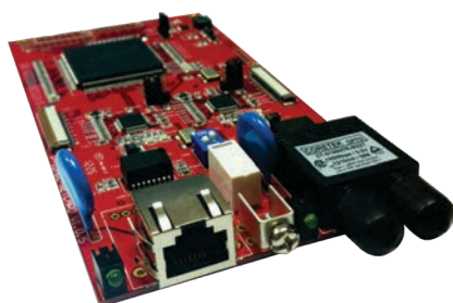
NET-C2, 1x RJ45 Port B i 1x fiber Port A
