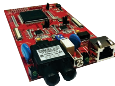
NET-C4, 1x fiber Port B i 1x RJ45 Port A
